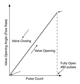
Output pulses change in the following orders when theValve is Closed $1 \rightarrow 2 \rightarrow 3 \rightarrow 4 \rightarrow 5 \rightarrow 6 \rightarrow 7 \rightarrow 8 \rightarrow 1$ Valve is Open $8 \rightarrow 7 \rightarrow 6 \rightarrow 5 \rightarrow 4 \rightarrow 3 \rightarrow 2 \rightarrow 1 \rightarrow 8$
