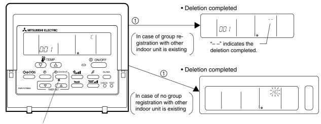
Press the switch for confirmation (F) twice continuously.
