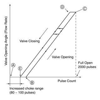
$\begin{array}{ll} \mbox{Output pulses change in the following orders when the} \\ \mbox{Valve is Closed} & 1 \rightarrow 2 \rightarrow 3 \rightarrow 4 \rightarrow 1 \\ \mbox{Valve is Open} & 4 \rightarrow 3 \rightarrow 2 \rightarrow 1 \rightarrow 4 \end{array}$
