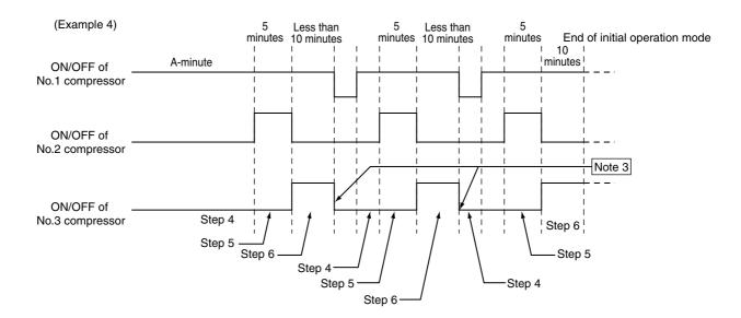
Note 1: If Step 4 is interrupted (compressor stopped by thermostat OFF or regular stop), Step 4 will be redone at restart.
